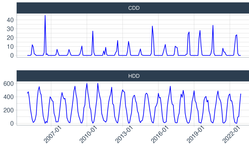
Figure F28: Cooling degree days and heating degree days, average across selected European countries.
